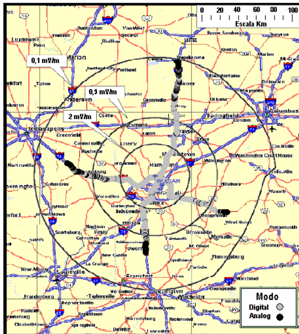
Testes NRSC - Freq. 1660 kHz - 10 kW
